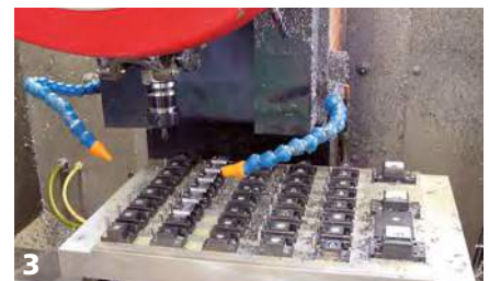
Picture 3. The use of a multiple workholding system is also beneficial in small batch machining
